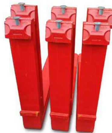
Higher specification fork mounting level-3B, more weight can be loaded.
