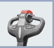
Simple and beautiful tiller designed to operate all functions easily even by one hand. Displayed turtle speed function applied to move slowly and helps to stack ponds in parrow spaces.
