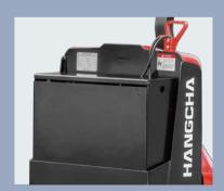
The battery compartment is sized to fit either a 12-85-5 industrial battery in its 7.8 inch compartmer for heavier throughout applications
